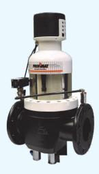
The PROFI and PROFIMAT allows water to flow and be filtered through a stainless steel filter sieve, which traps and retains all the physical impurities until an automatic backwash is initiated. During backwash there is NO interruption to the buildings water supply or to the filtration process due to the working principals of the filters patented backwash point-rotation-system allowing water to be filtered even during a backwash cycle.
